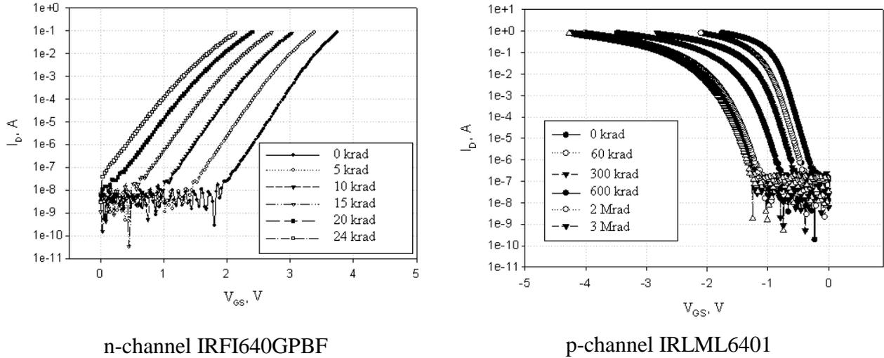
Fig. 2. Power MOSFETs total dose degradation
