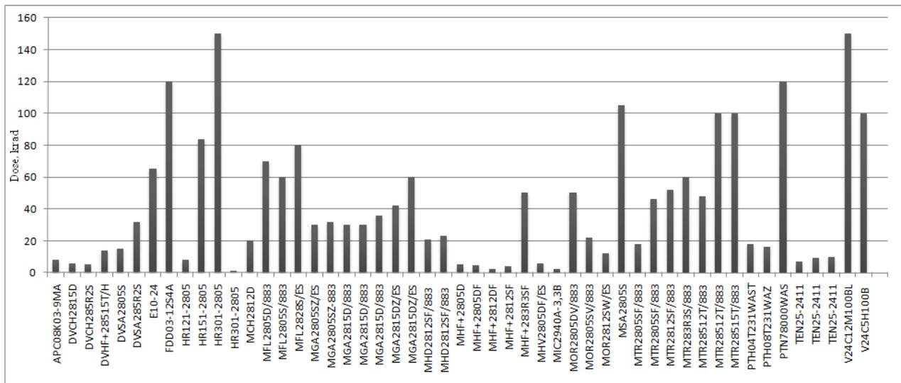
Fig. 1. Experimentally obtained DC-DC converters total dose hardness levels
