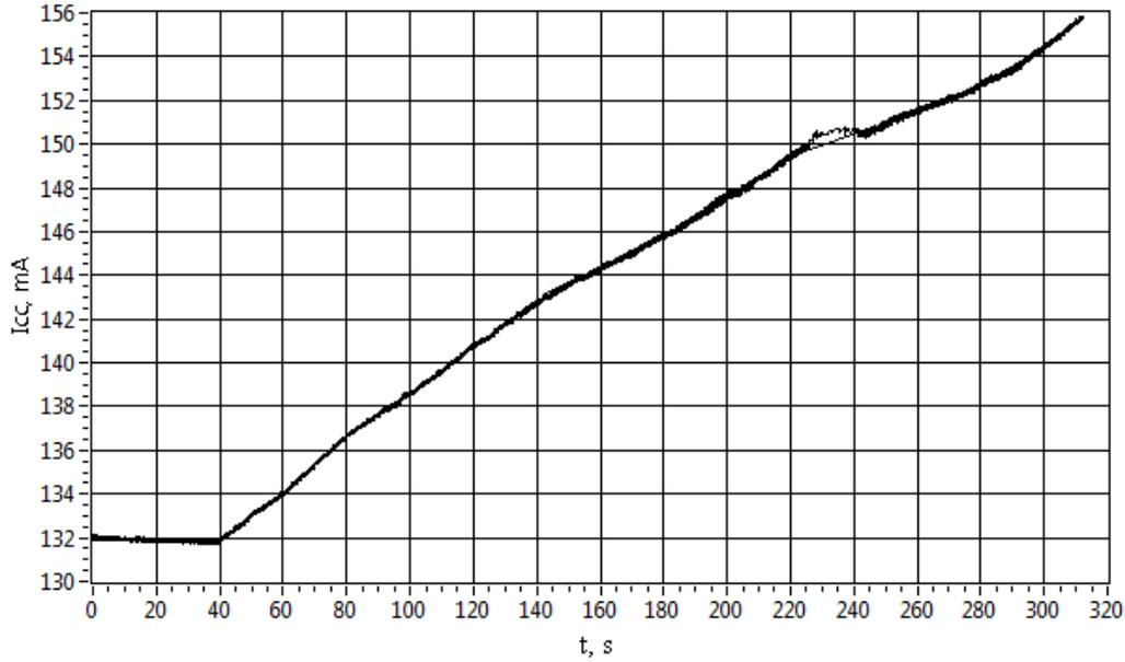
Fig.3. PTH03060WAH supply current vs. time during Xe-ion irradiation (only MOSFET is irradiated)
