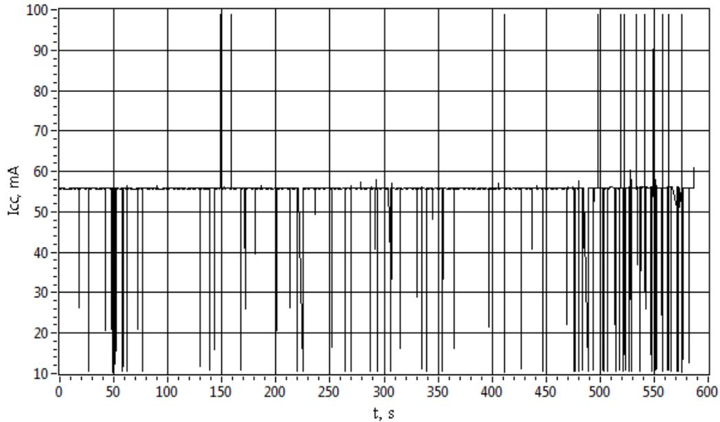
Fig.4. PTH03060WAH supply current vs. time during Xe-ion irradiation (only PWM is irradiated)
