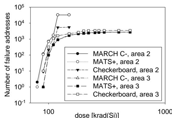
Fig. 4. Number of failure addresses in FRAM vs total dose.
