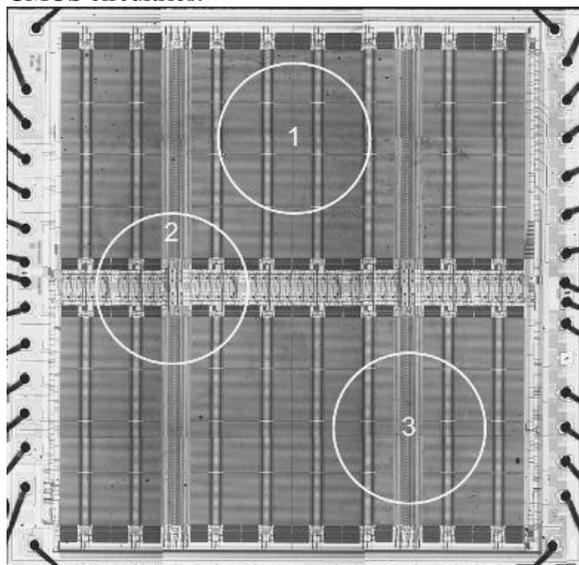
Fig.1. Areas on the dies FM18L08, which were irradiated through the shield.
