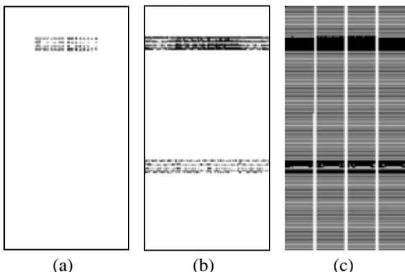
Fig. 2. Physical positions of the failing bits (black points) in FRAM FM18L08 irradiated through the shield with a hole at area 2: (a) 90 krad(Si), (b) 110 krad(Si), (c) 120 krad(Si).
