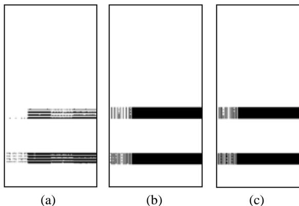
Fig. 3. Physical positions of the failing bits (black points) in FRAM FM18L08 irradiated through the shield with a hole at area 3: (a) 250 krad(Si), (b) 270 krad(Si), (c) 500 krad(Si).
